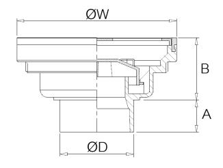
Medium - heavy duty residential applications . Furnished with ABS body and stainless steel grate. Fit for pipe  $\varnothing 2$ " to  $\varnothing 3$ "
