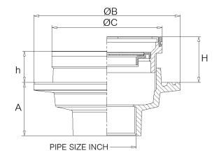
Medium - heavy duty residential applications . Furnished with ABS body and stainless steel grate. Fit for pipe  $\varnothing 2$ " to  $\varnothing 4$ "
