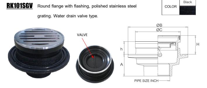
Medium - heavy duty residential applications . Furnished with ABS body and stainless steel grate. Odor protection by batterfly gravity valve. Fit for pipe  $\emptyset 2$ " to  $\emptyset 4$ "
