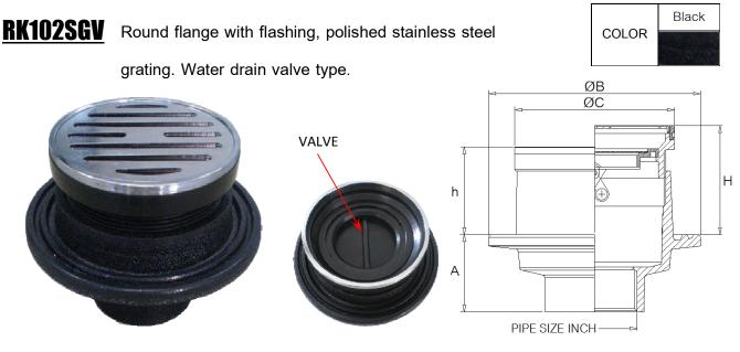
Medium - heavy duty residential applications . Furnished with ABS body and stainless steel grate. Odor protection by batterfly gravity valve. Fit for pipe  $\emptyset 2$ " to  $\emptyset 4$ "
