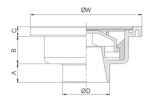
Light duty residential applications this drain is furnished with ABS body and ABS grate. And odor protection by water trap. Fit for pipe inside  $\varnothing 1.5$ " to  $\varnothing 3$ "
