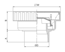
Light duty residential applications this drain is furnished with ABS body and square plastic tray . And odor protection by water trap. Fit for pipe inside  $\varnothing$  2" to  $\varnothing$  4".
