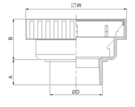
Light duty residential applications this drain is furnished with ABS body and ABS grate. Fit for pipe inside  $\varnothing$  2" to  $\varnothing$  4" .
