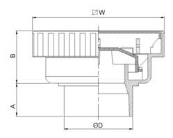
Light duty residential applications this drain is furnished with ABS body and stainless steel grate. And odor protection by water trap. Fit for pipe inside  $\varnothing$  2" to  $\varnothing$  4"
