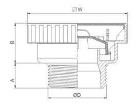
Light duty residential applications this drain is furnished with ABS body and stainless steel grate. And odor protection by water trap. Fit for connector pipe PT 2" and PT 3"
