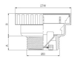
Light duty residential applications this drain is furnished with ABS body and stainless steel grate. And odor protection by sealing valve. Fit for connector pipe PT 2" and PT 3".
