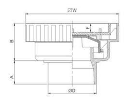
Light duty residential applications this drain is furnished with ABS body and square tray with ceramic style. And odor protection by water trap. Fit for pipe inside  $\varnothing$  2" to  $\varnothing$  4".
