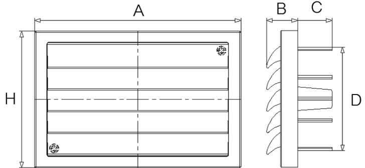
ABS body with UV protection. 5 curve blade with insect protection net. Suitable for dry exhaust air. Especially from bathroom, kitchen and drying machine. Can be Installed with both Flexible foil duct 4 "and Square duct 3" x 6 " or 4" x 6 "
